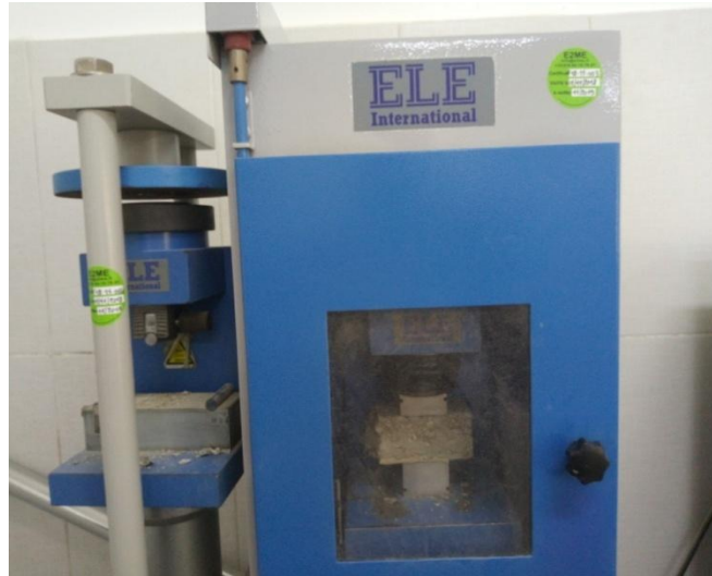
FIG. 4 The bending and compression testing equipment
