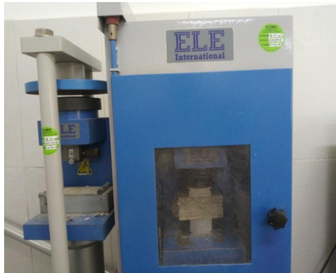
FIG. 4 The bending and compression testing equipment
