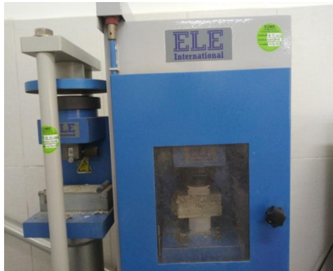
145 FIG. 4 The bending and compression testing equipment
