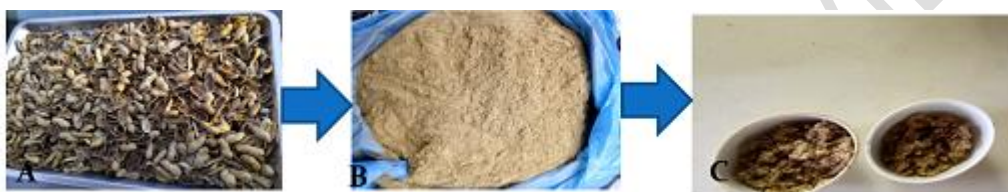
Fig 1. A: Groundnut shells B: pulverized Groundnut shells C: Groundnut Shell Coagulant (GSC)
