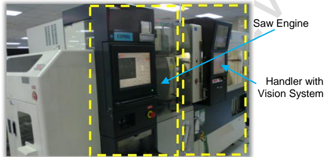
Fig. 2. Package singulation machine with integrated Handler and Vision system
