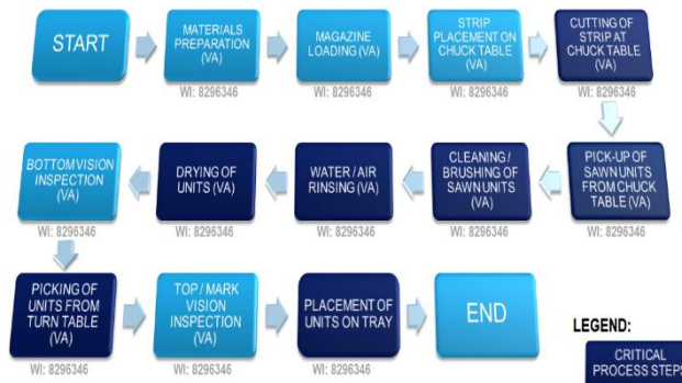
Fig. 5 Package Singulation: a Detailed Process Flow
