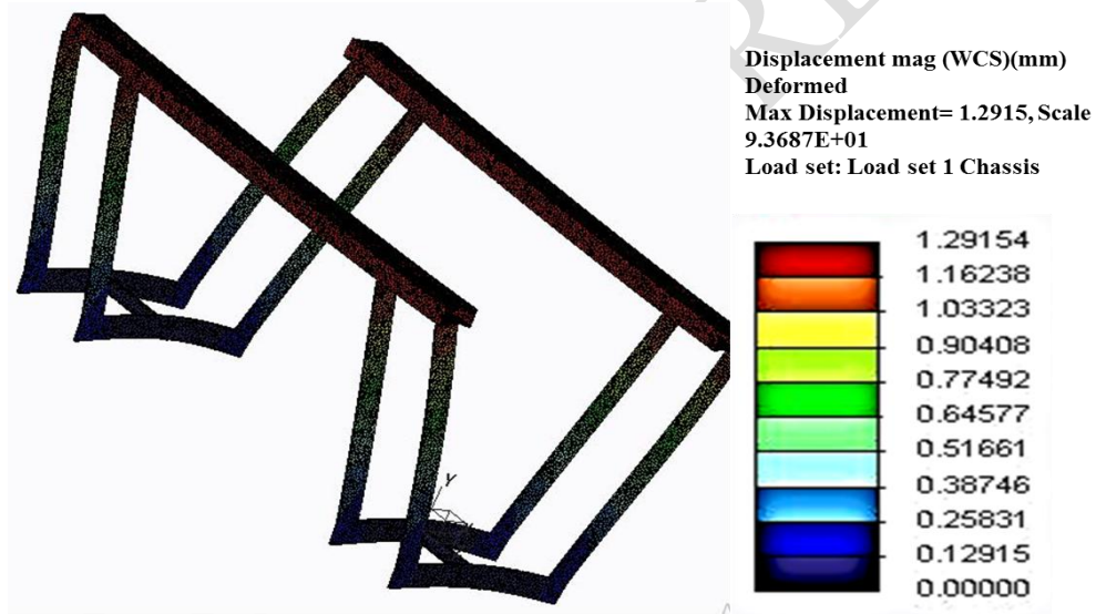
Fig.13 Displacement analysis on Sub-frame assembly
