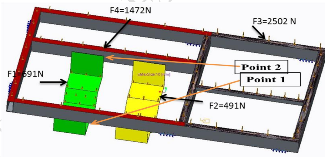
Fig. 6 Boundary conditions in Chassis
