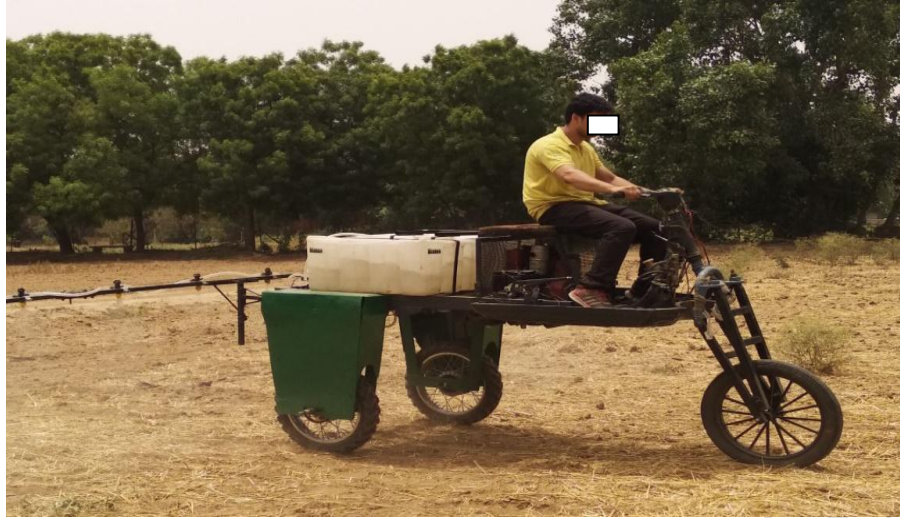
Fig.15 Actual prototype of high clearance foliar applicator
