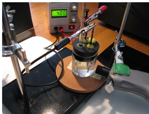
Figure 1. HyPIR Electrolysis Apparatus (courtesy Fanchi Enterprises)
