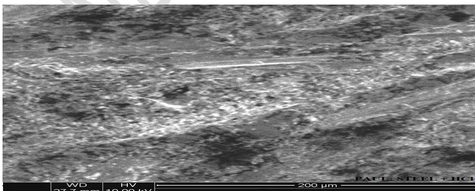
Figure 6: SEM image of pipeline steel in 0.5 M HCl without CCC aqueous extract
