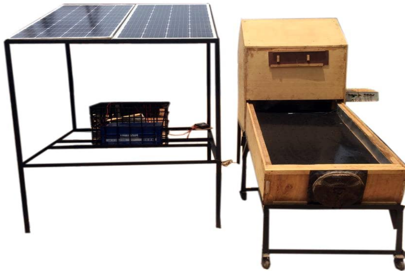
FIGURE 3. The developed solar controlled hot-air supplemented dryer.
