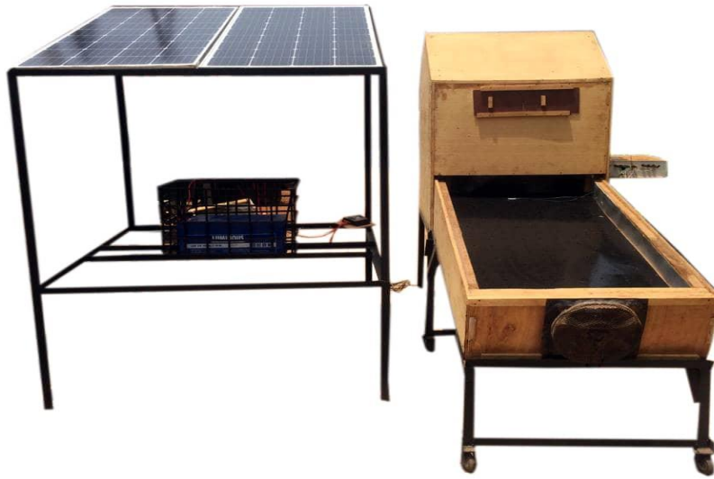
FIGURE 3. The developed solar controlled hot-air supplemented dryer.
