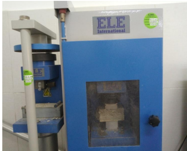
FIG. 4 The bending and compression testing equipment
