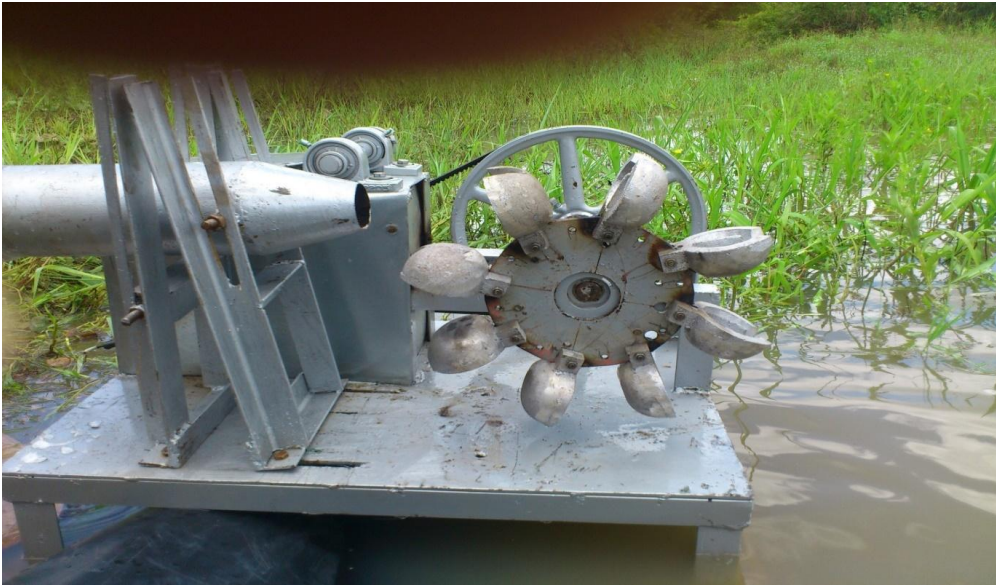
Figure 2: Pictorial view of the Pelton Wheel Turbine
