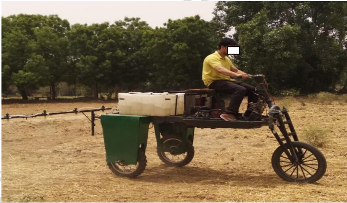
Fig.15 Actual prototype of High clearance foliar applicator
