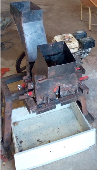
Fig. 2. Operating the dual compartment ginger slicing machine
