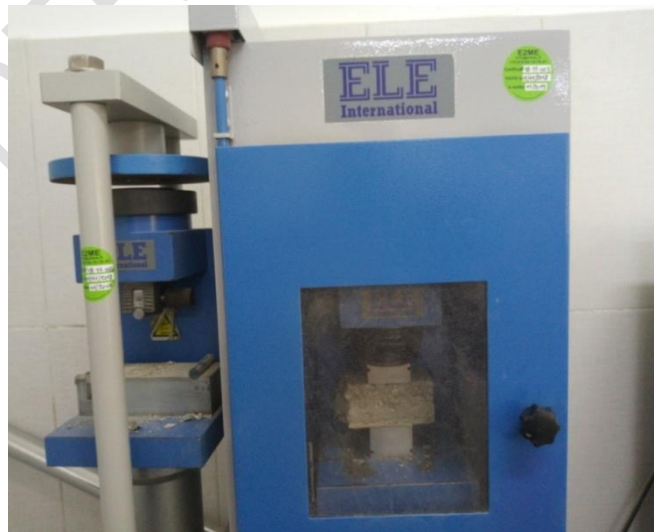
Fig. 4: The three-point bending and compression testing equipment on the test specimen
