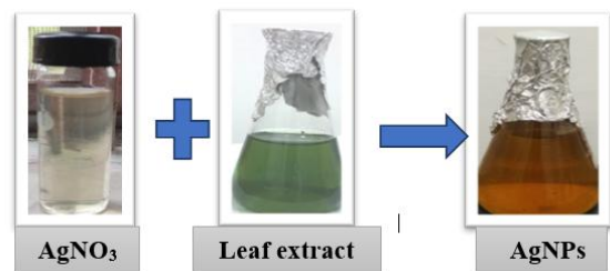
Fig 2: Pictures show the visual identification Of AgNPs synthesis by A.paniculata leaf extract.
