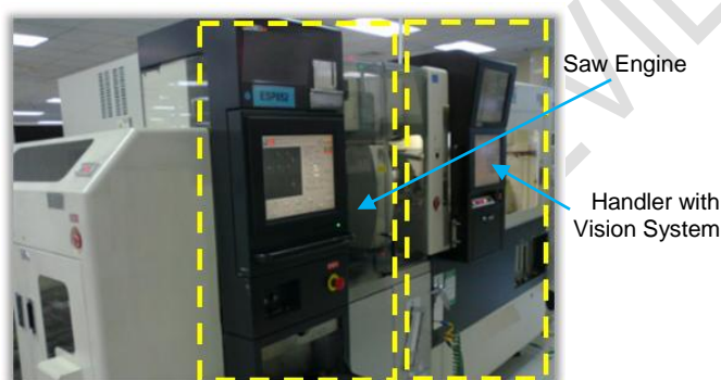
Fig. 2. Package singulation machine with integrated Handler and Vision system
