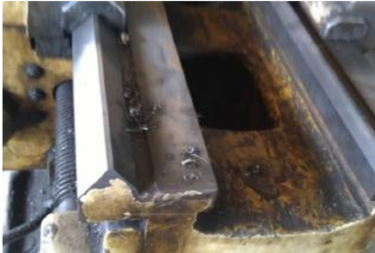
Conventional lathe dovetail guide way and saddle [12]
