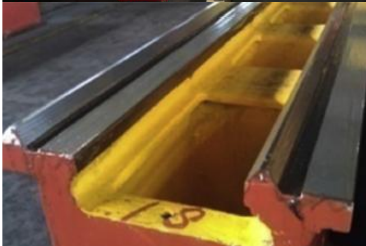
Fig.7. Insert/mate/screw ball linear guide based assembly and dovetail guide way based remanufactured [11][12].
