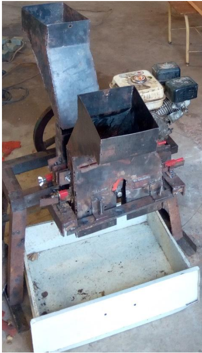
Fig. 2. Operating the dual compartment ginger slicing machine
