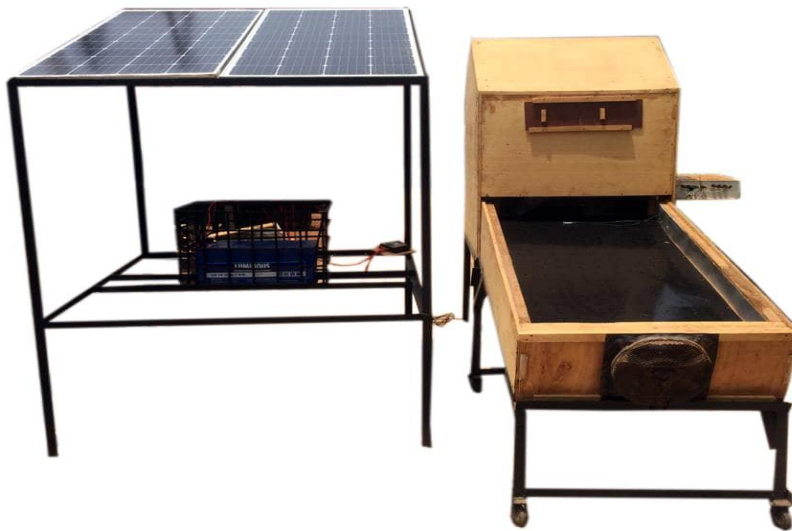
327 Figure 3: The developed solar controlled hot-air supplemented dryer
