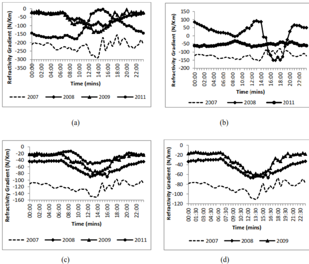
Fig. 3. Diurnal Variation of refractivity gradient for a typical day during the rainy season at (a) 50 m (b) 100 m (c) 150 m (d) 200m (July 2nd) from 2007 – 2009 and 2011
