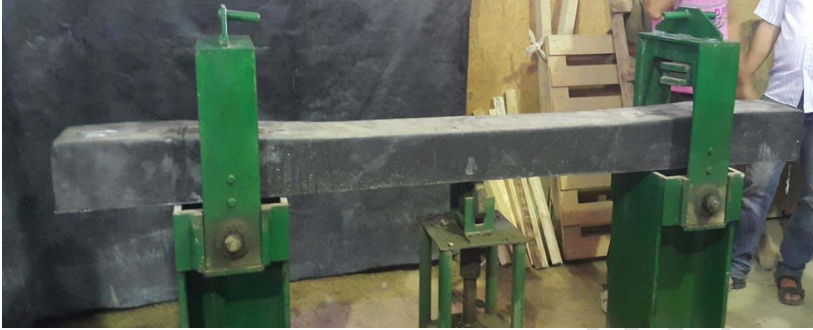
Fig.5. Actual set up of negative bending test at center of sleeper
