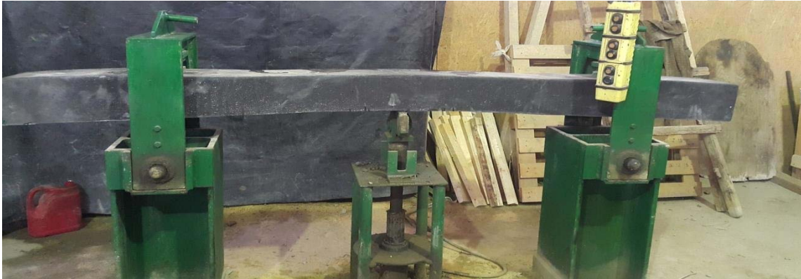
Fig.9. Sleeper (S 10 ) under 72 kN static loading of the sleeper center section.
