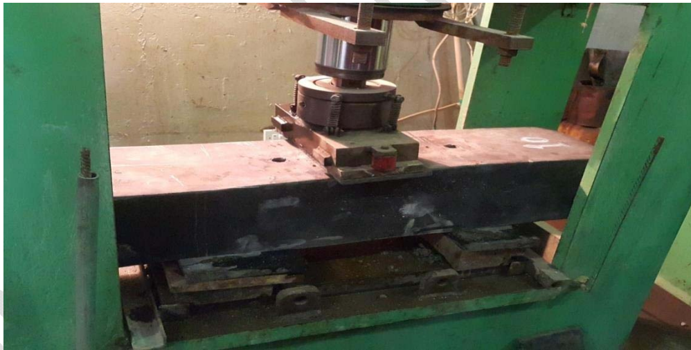
Fig.7. Actual set up of positive bending test at rail seat position
