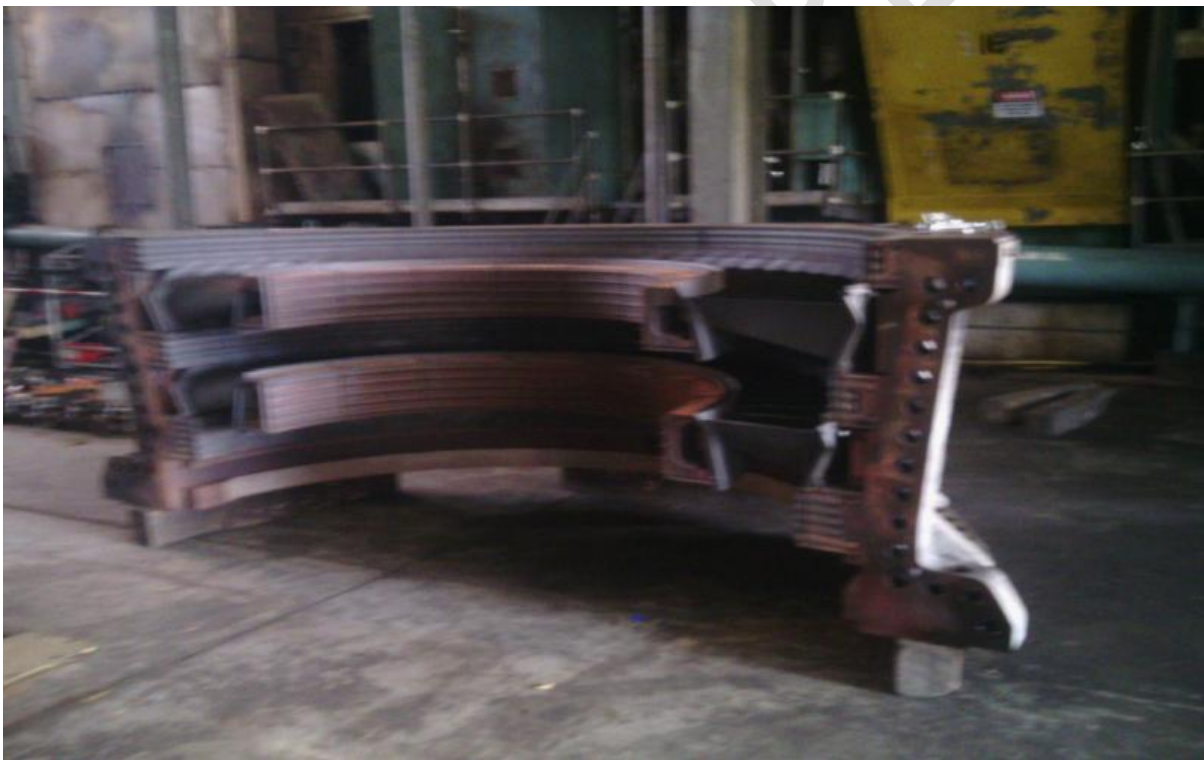
FIG.21: COUPLING OF NOZZLE TO THE SHROUD.
