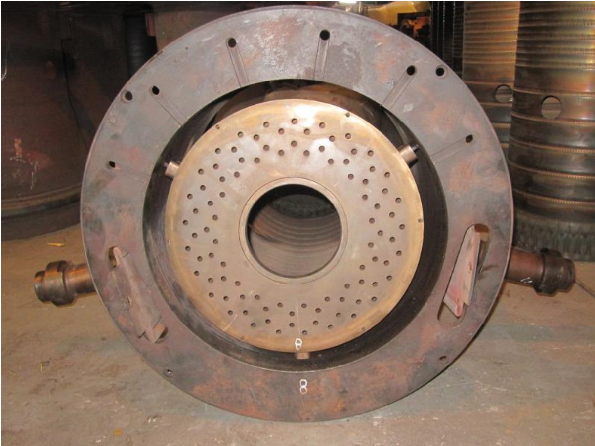
Fig. 17. Linear/flow sleeve/transition piece/cross-fire tube Assemble. (Front view)
