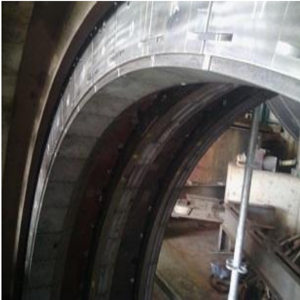
Fig. 19: coupling of shroud block
