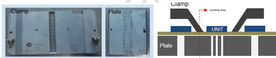
Fig. 5. Wirebond process plate design (landing area)
