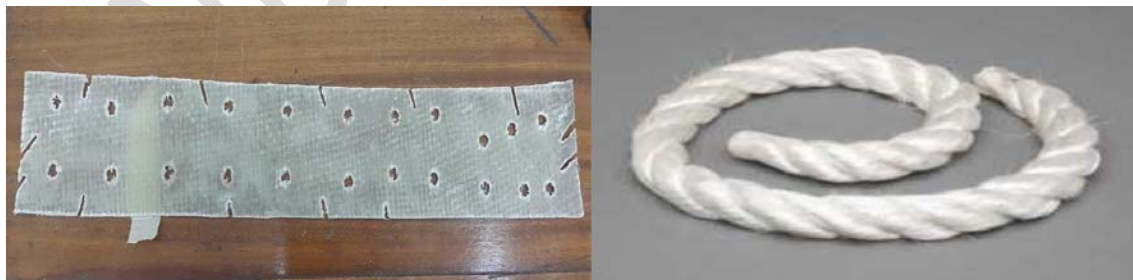
Fig.3. used fiber glass laminate and rope in sleeper reinforcement
