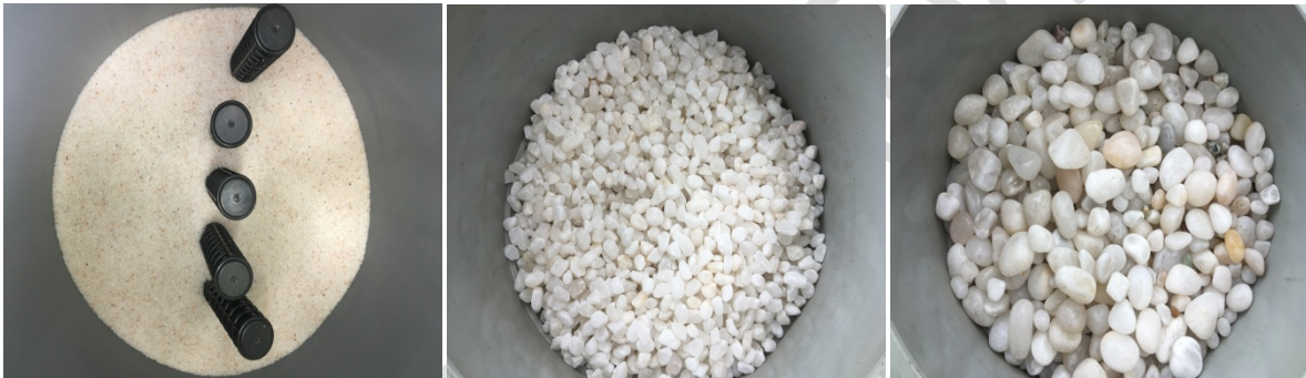
Fig.4. Layers of sand, gravels and pebbles
