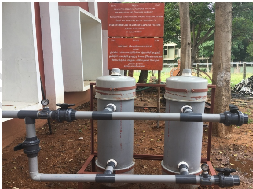
Fig. 5. Developed Double Chamber Low Cost Filter
